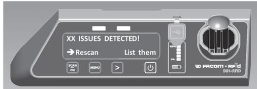
⇒ The user can then run a new scan to check there is no error (see 'Characteristics, general information & Warnings' section), or list the missing tool(s). The selection is made using the arrow button.
