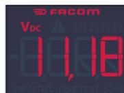
If a default is identified the LCD screen goes red with an alarm.
