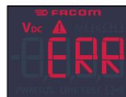
If the DX.V12 is used on higher than 49V volt circuit a error «ERR» is show with an alarm.
